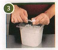
Adjust the thermometer so it reads 32°F (0°C).
